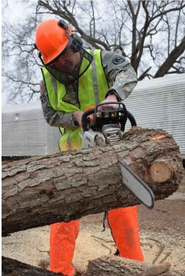
Mesh face shield worn during chainsaw work. (*6)
