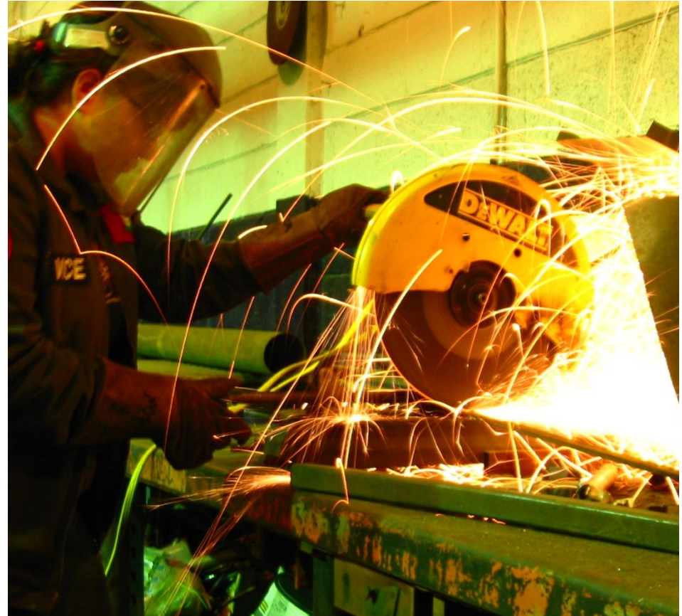
Worker wearing eye protection and face shield for welding/cutting activity. (*1)
